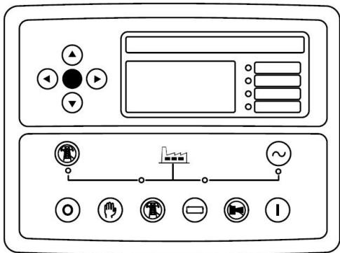
The DSE7310 MKII is an Auto Start Control Module and the DSE7320MKII is an Aut Mains (Utility) Failure Control Module suitable for a wide variety of single, diesel or gas, gen-set applications.
